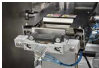
Cross sealing jaws with stripping action
