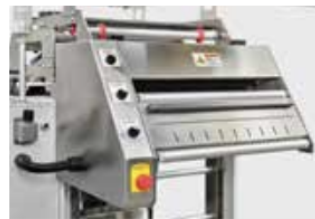
Servo driven Unwinding with splicing plate
