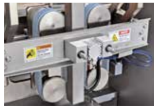
Vacuum assisted Bag pulling system
