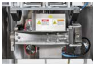
Bag pulling system
